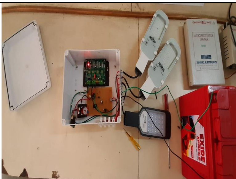
D ) DC-DC Converter assembly, with batteries and LED Lamps during testing in the laboratory of EEE department at AVIT.
