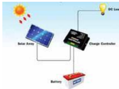
Fig. 6.1. Stand alone PV system
