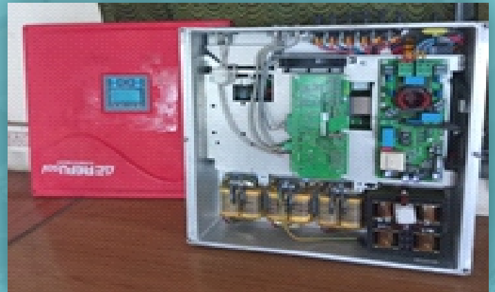
Inverter control testing for different operating conditions
