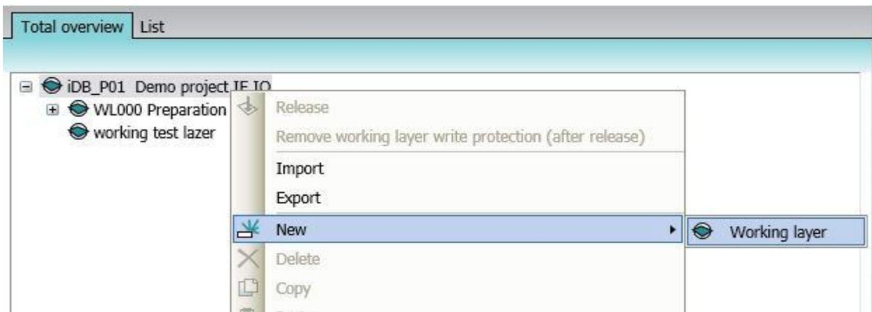
The new window will be open in that you can give name for the working layer and give OK the working layer created. The below shown image you can create name for the working layer.
