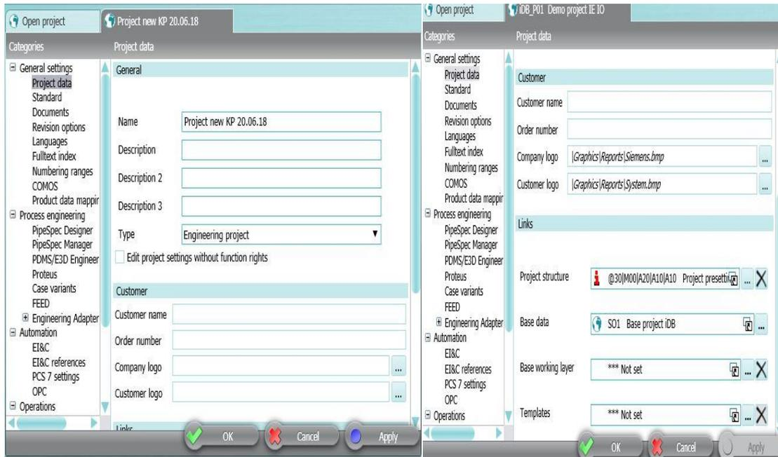
STEP 6: Now select the project structure with respect to the need we can select the project structure from the listed structures as show in below
