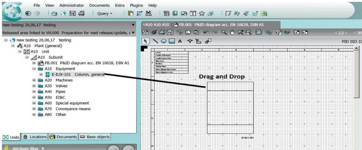
All the Equipments, Instruments, valves and special machines are can be used in the working area by drag and drop method.
