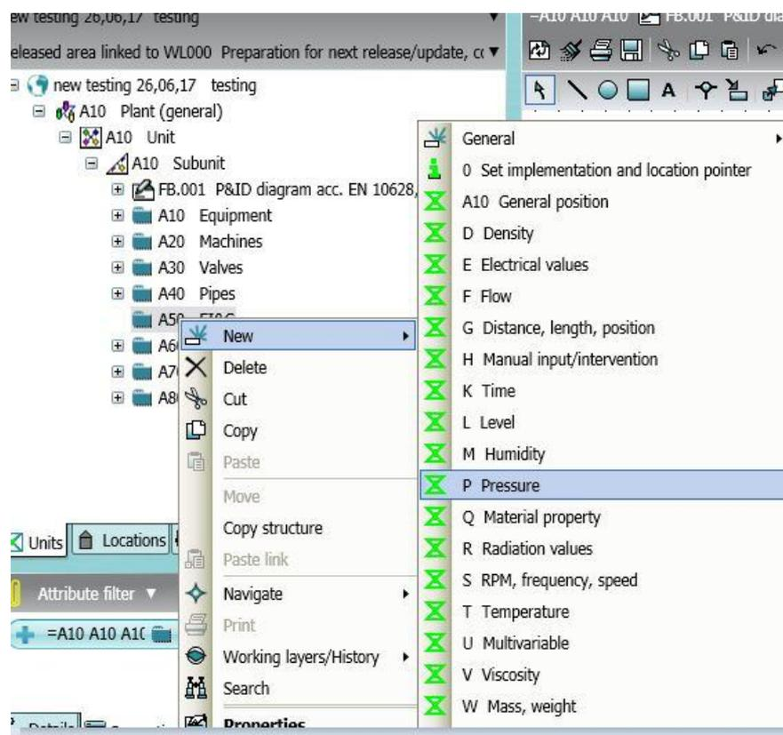
From shown above image we can create the require instruments. And again select the Pressure and go to new and give pressure as shown in below.
