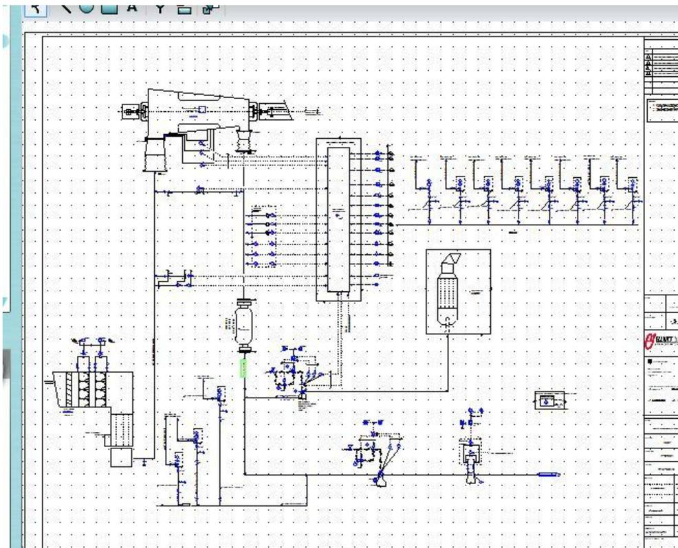
The P&ID diagram would be like above image. All the equipments and instruments which are used in this above Piping and Instrumentation Diagram are created by context menu.
