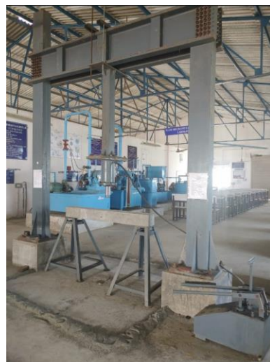
Loading Frame - 50 Tonne capacity
