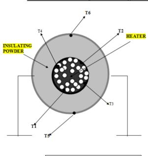
DIAMETER OF INNER SPHERE = 76mm
