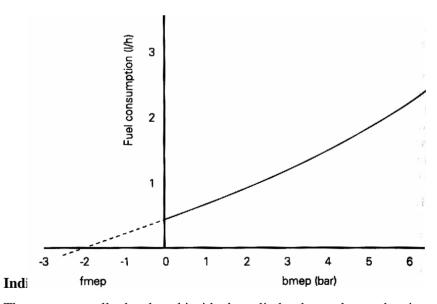
The power actually developed inside the cylinder due to the combustion of fuel is called indicated power .
