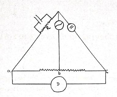
The cell "A" is in the one arm and resistance box "R" constitutes the other arm, the source of alternating current is represented as "S" and "ad" is calibrated slide wire of uniform resistance and "D" is current detectors.
